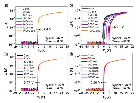
Figure 8. Evaluation of device transfer curves with (a,c) four and (b,d) eight hydrogen barrier cycles under PBTS ( $V_{gstr} = 20$  V, Temp. = 60 °C) and NBTS ( $V_{gstr} = -20$  V, Temp. = 60 °C).
