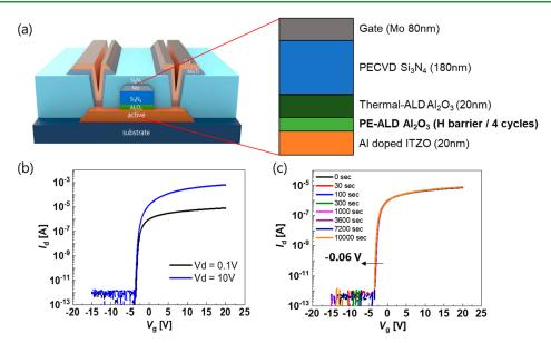
Figure 11. (a) Schematic of the self-aligned TFT with a hydrogen barrier. (b) Transfer curve of the self-aligned TFT with four hydrogen barrier cycles. (c) Overlapped transfer curve under PBTS of over 10 000 s.
