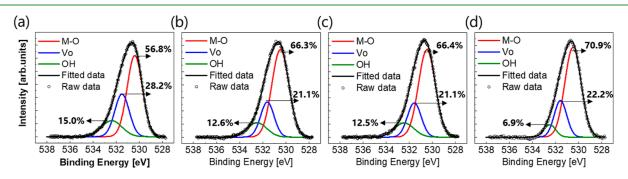
Figure 7. Spectra of XPS O 1s for the active layer surface (a) without additional barrier, (b) with two cycles, (c) four cycles, and (d) eight cycles of the barrier.
