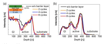
Figure 5. Depth profiles of (a) H and (b) OH in the GI/active/substrate structure with different H barrier thicknesses.
