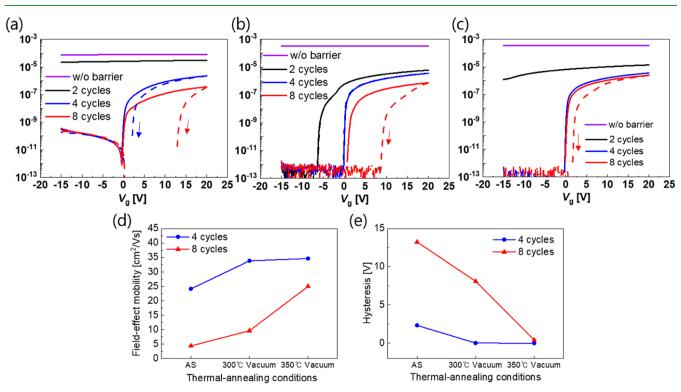
Figure 2. Transfer characteristics of TFTs with different thicknesses of barrier conditions: (a) before annealing, (b) after vacuum annealing at 330 °C, and (c) after vacuum annealing at 350 °C. The trends of (d) field-effect mobility and (e) hysteresis are based on the thermal annealing temperature.
