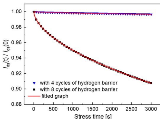
**Figure 9.** Decay of the normalized drain current during bias stress and fitted curves with stretched exponential formulas.
