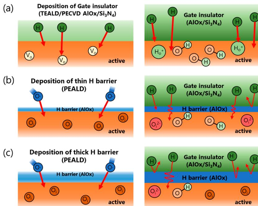
Figure 6. Illustration of a possible hydrogen incorporation mechanism in the case of (a) without an additional barrier and (b) with thin and (c) thick hydrogen barrier deposition processes.
