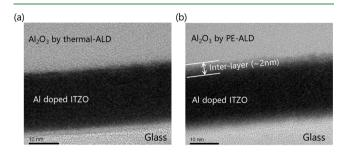
Figure 3. HRTEM images of cross-sectional film stacks with  $Al_2O_3$  deposited by (a) thermal-ALD and (b) PE-ALD.
