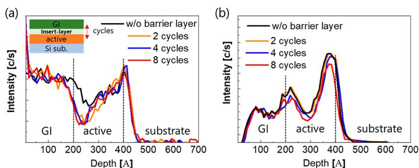
Figure 5. Depth profiles of (a) H and (b) OH in the GI/active/substrate structure with different H barrier thicknesses.
