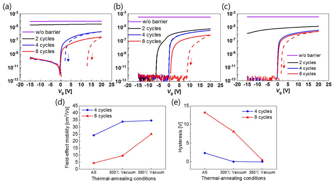
Figure 2. Transfer characteristics of TFTs with different thicknesses of barrier conditions: (a) before annealing, (b) after vacuum annealing at 330 °C, and (c) after vacuum annealing at 350 °C. The trends of (d) field-effect mobility and (e) hysteresis are based on the thermal annealing temperature.
