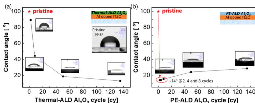
**Figure 4.** Contact angle variation on the oxide semiconductor surface with cycles of (a) thermal-ALD and (b) PE-ALD for Al<sub>2</sub>O<sub>3</sub> layer deposition. The inset indicates the contact angle of the pristine oxide semiconductor.
