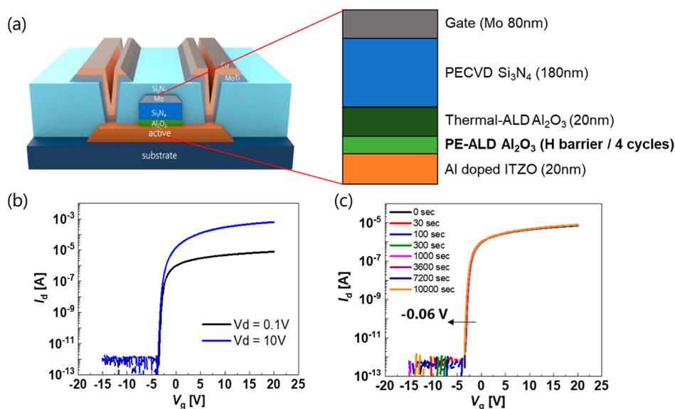
**Figure 11.** (a) Schematic of the self-aligned TFT with a hydrogen barrier. (b) Transfer curve of the self-aligned TFT with four hydrogen barrier cycles. (c) Overlapped transfer curve under PBTS of over 10 000 s.
