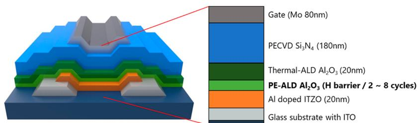
Figure 1. Schematic of a high-mobility TFT with an ultrathin hydrogen barrier layer.
