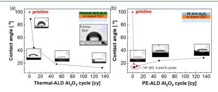
**Figure 4.** Contact angle variation on the oxide semiconductor surface with cycles of (a) thermal-ALD and (b) PE-ALD for  $Al_2O_3$  layer deposition. The inset indicates the contact angle of the pristine oxide semiconductor.
