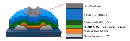
Figure 1. Schematic of a high-mobility TFT with an ultrathin hydrogen barrier layer.
