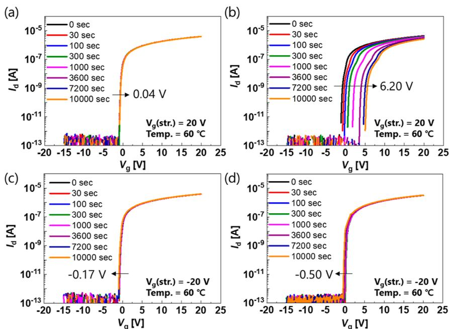
**Figure 8.** Evaluation of device transfer curves with (a,c) four and (b,d) eight hydrogen barrier cycles under PBTS ( $V_{g,\text{str}} = 20$  V, Temp. =  $60$  °C) and NBTS ( $V_{g,\text{str}} = -20$  V, Temp. =  $60$  °C).
