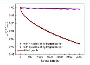
**Figure 9.** Decay of the normalized drain current during bias stress and fitted curves with stretched exponential formulas.
