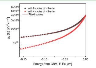
Figure 10. Subgap states of the devices derived using the DIFT based on the hydrogen barrier conditions.
