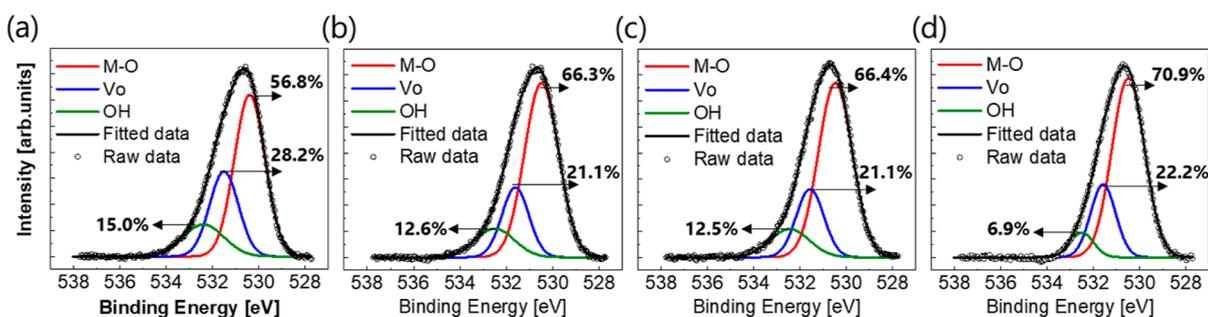
Figure 7. Spectra of XPS O 1s for the active layer surface (a) without additional barrier, (b) with two cycles, (c) four cycles, and (d) eight cycles of the barrier.
