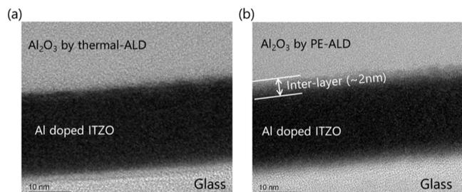
**Figure 3.** HRTEM images of cross-sectional film stacks with Al<sub>2</sub>O<sub>3</sub> deposited by (a) thermal-ALD and (b) PE-ALD.
