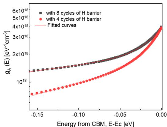
**Figure 10.** Subgap states of the devices derived using the DIFT based on the hydrogen barrier conditions.
