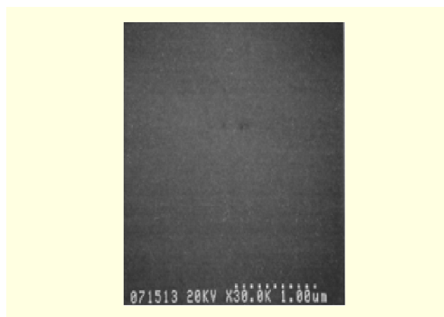
Fig. 1. SEM image of \text{AlO}_x thin film deposited at 80°C using 500 cycles.
